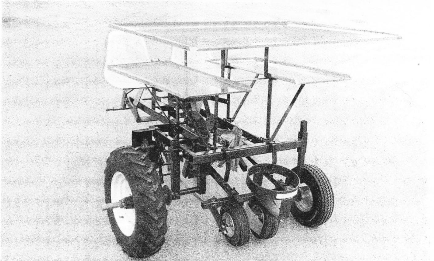
PHOTO SHOWS PLANTER WITH STANDARD SINGLE WHEEL DRIVE AND IDLER WHEEL, AND OPTIONAL FULL TOP TRAY
