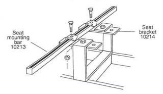
Attach the seat mounting bar (10213) to the seat bracket (10214) as shown. Secure with the 1/2" x 2" carriage bolts, bent seat washers and 1/2" nuts. The seat bracket can be adjusted forward or backward on the unit frame for maximum operator comfort. Attach the seats to the mounting bar as per the instructions supplied with the specific type of seats you purchased. Make sure all bolts and nuts are securely fastened before allowing anyone to sit on the transplanter.
