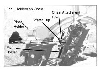
Secure with the 5/16" nut (see illustration). Make sure the plant holder is perpendicular to the chain before tightening. The water trip is not necessary for planting units that do not have a water valve attachment. Adjust upper conveyor pulley by tightening or loosening the pulley bolts to make plant holders travel through center of closing guides. To avoid damage, never run plant holders through the guides in reverse direction.
